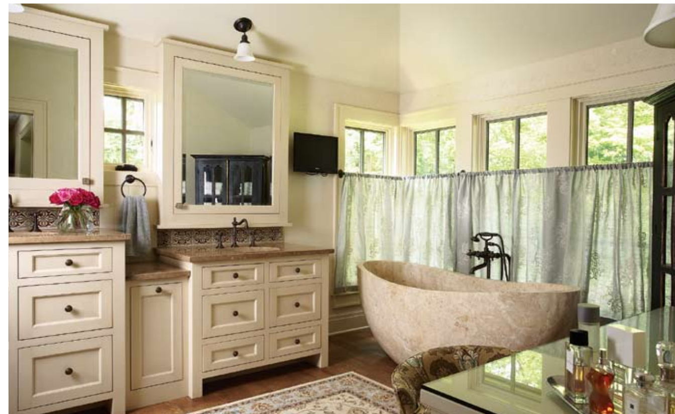
The owners' bath features his-and-her vanities, built to order for the tall husband and short wife. But the star here is the 1,500 pound travertine tub. It required extra bracing in the floor and customized plumbing for the faucets.
